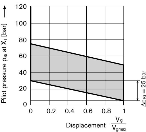
**H3**  $\Delta p_{st}$  for hydraulic stroke limitation \_\_\_\_\_ 35 bar
