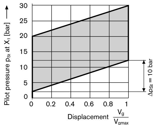
**N2**  $\Delta p_{st}$  for hydraulic stroke limitation \_\_\_\_\_ 25 bar
