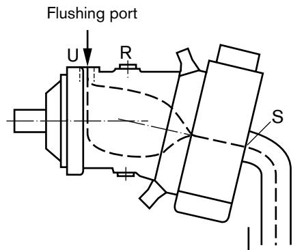
Flushing flows for A7VO same as bearing flushing
