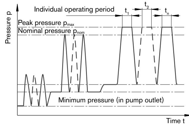
Total operating period =  $t_1 + t_2 + \dots + t_n$
